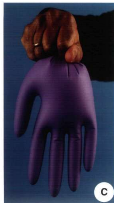
A simple method for detecting fine holes in a glove. A - stretch the cuff of the glove, trapping a small amount of air inside. B - fold the cuff over several times to compress the air. C - if the glove is hole-free, it should remain inflated like this.
